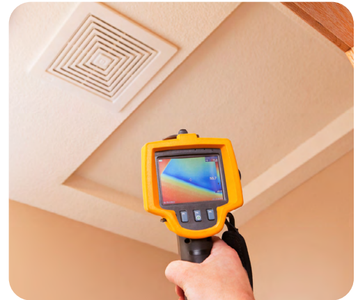
An infrared thermal camera, held by a Registered Energy Advisor's hand, is pointed at a ceiling vent.
