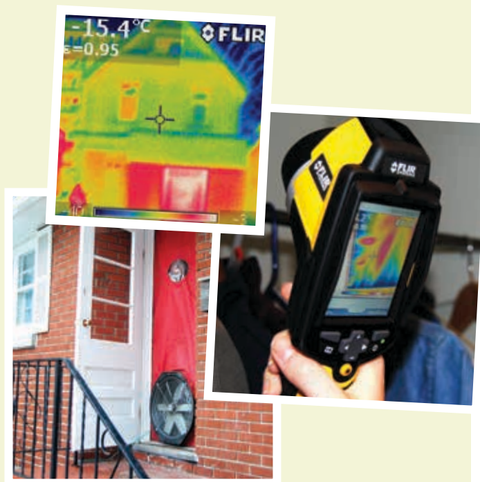
A blower door is used to measure air leakage in the house. Used with a blower door test, an infrared camera visually enhances the detection of air leaks.
